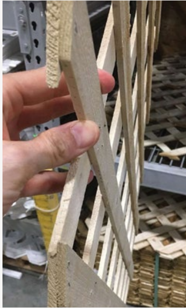
Big Box retailer's lattice Pine wood 1/4" thick
