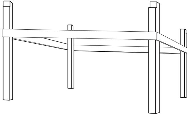
Reattach the fourth side of the template and make sure all posts are square and plumb.
