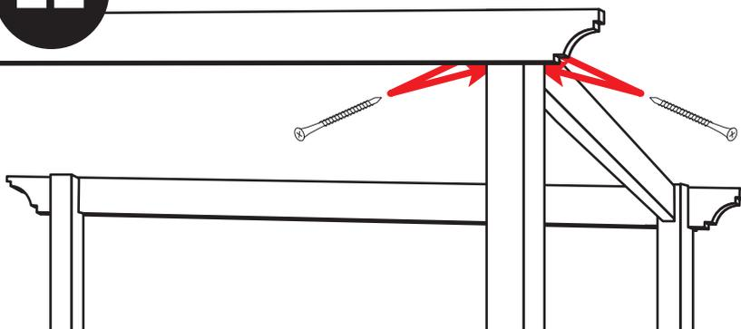
While the return beam is being held on both ends between the high side and the low side. Attach to the high side first, being sure to center the beam in the middle of the post and making the top of the beam flush with the top of the post. Attach with four 3 1/2" screws, two per side.
