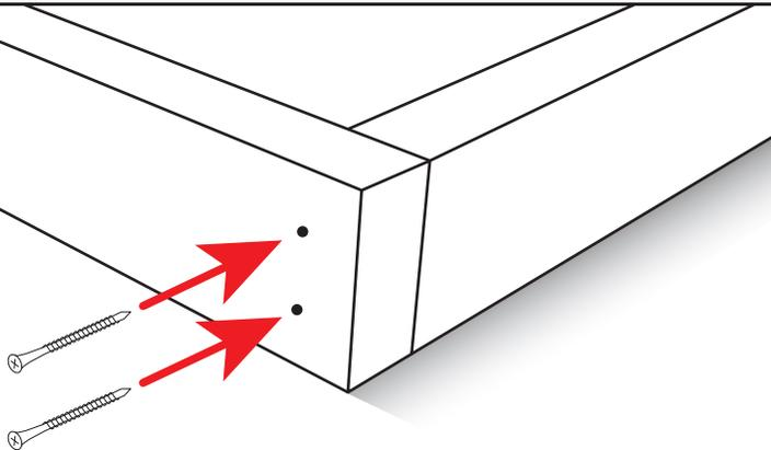
Connect the corners of the template pieces by driving two 2 1/2" screws through the side of the template boards.
