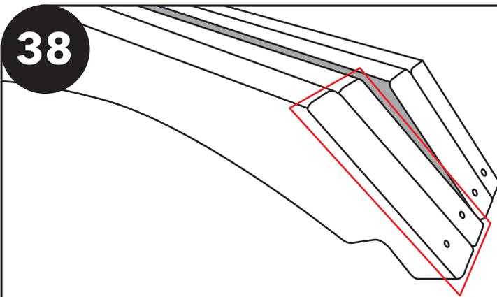
Locate the four braces with different angles cut on the top and bottom. based on the angles cut. **NOTE: When installing, if both ends are not flush before drilling, do not install. Find the brace that fits the angle.** For pressure treated, be sure brace side screws are facing inside the pavilion.
