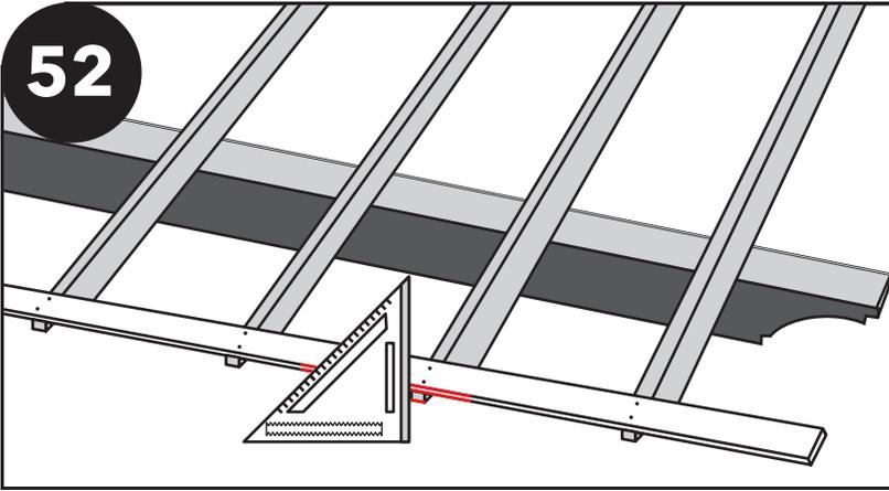
**VERY IMPORTANT:** Be sure first decking board is flush with the ends of the rafters, so the remaining boards attach squarely.
