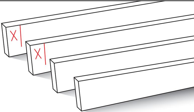
The Pavilion kit includes a wooden template that will be used to mark the post locations. Notice that two of the 2x4 boards have a marking near the ends. Building a box will reveal the outside corners of the posts when properly placed.
