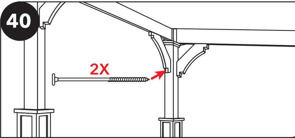
Keeping the brace centered on the post, attach the brace into the post through the pre-drilled holes with the 5" Timberlock screws.
