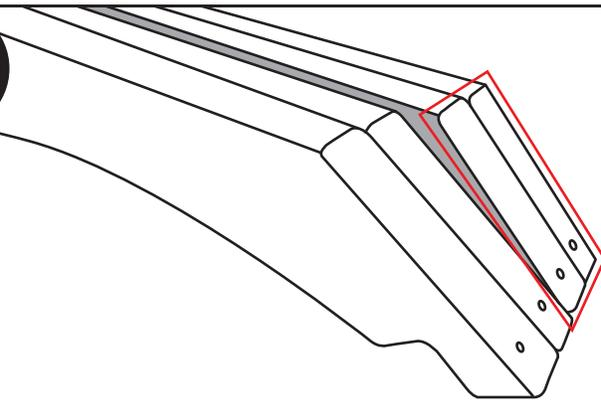
Lay them on the ground and choose the four braces that have the same angle at the top and the bottom. These will be used to support the two main headers (Front and back).
