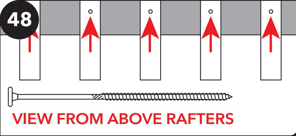
Attach the rafters into the low side header from the top down with one 8" GRK screw.
