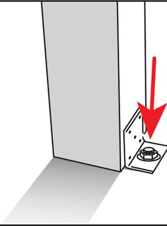
Once the wedge anchor is down against the bracket use a wrench and tighten it. Do that with all the anchors.
