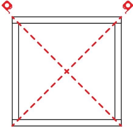
Once the template is in position, square the template. Do this by measuring diagonally from one corner to its opposite corner, then measure diagonally between the other two corners. These two dimensions **MUST** be the same. Adjust the template until the diagonal measurements are identical.
