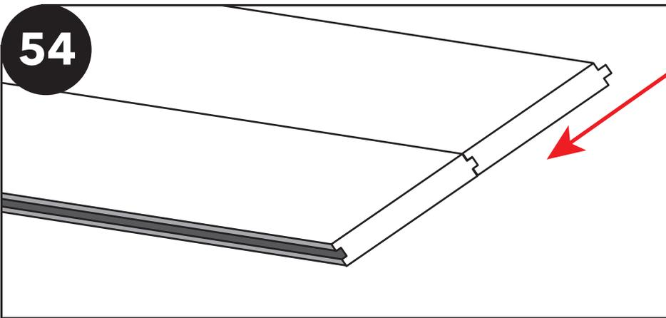
Tightly fit the next boards groove into the installed tongue board. **NOTE:** Be sure board is fully seated before screwing into place.
