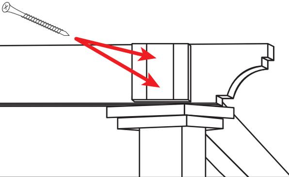
Locate header trim piece (4 total), center the first piece above top trim on the outside of the header and attach with two 2 1/2" screws. Repeat on all remaining posts on the outside of the header.
