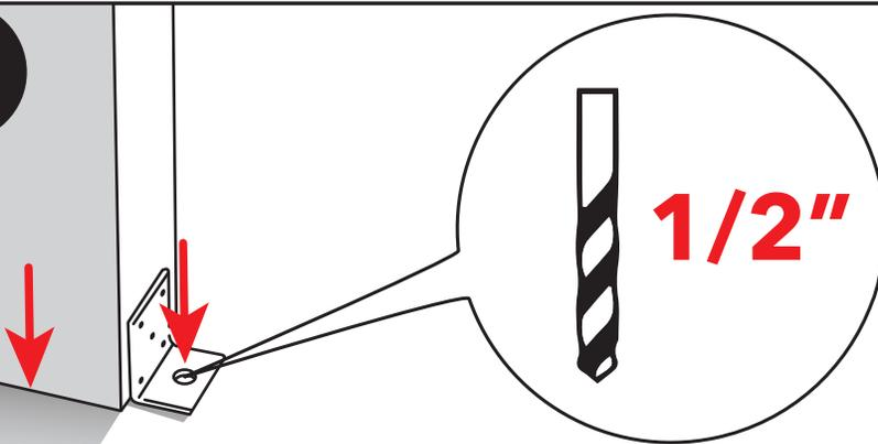
When all posts have an L bracket on, use a drill with 1/2" masonry bit to drill down about 1/2" farther than length of wedge anchor.
