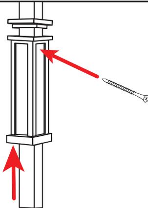
Slide post bases up 3' and attach with one 2 1/2" screw to hold in place."
