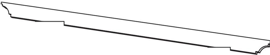
Locate the 2x6 rafters. The number of rafters will vary based on length of pavilion. Rafters will be notched on bottom in two places to sit flush on the top of header.
