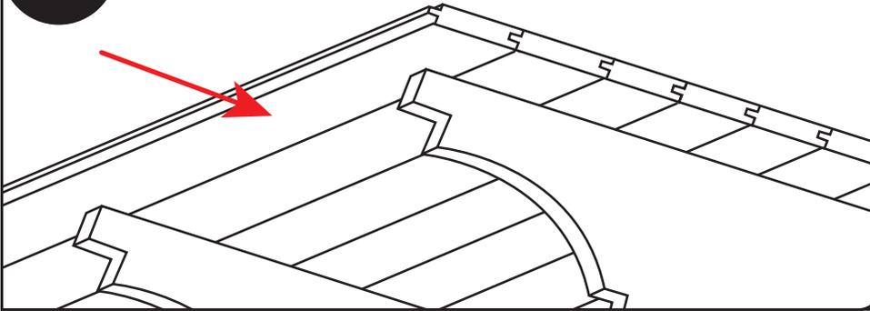
Fit last decking board tightly into place, but do not fasten. This board will completely cover all rafter ends.
