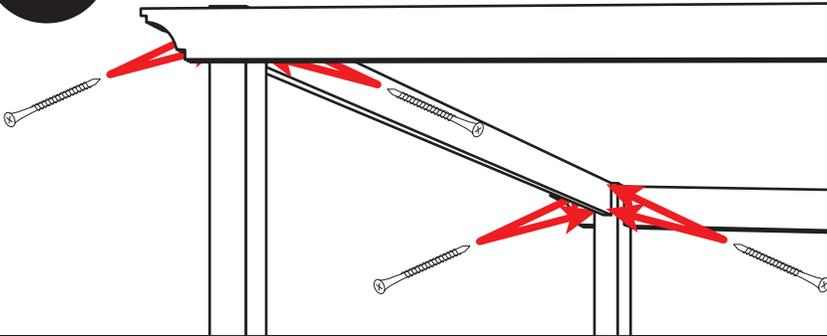
To finalize return beam installation, locate the eight 8" GRK screws. Send two GRK screws from the outside of the header into the return beams, using the pre-drilled holes. Repeat on all four posts.
