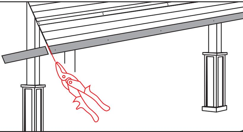
Using tin snips, cut drip edge accordingly. a
