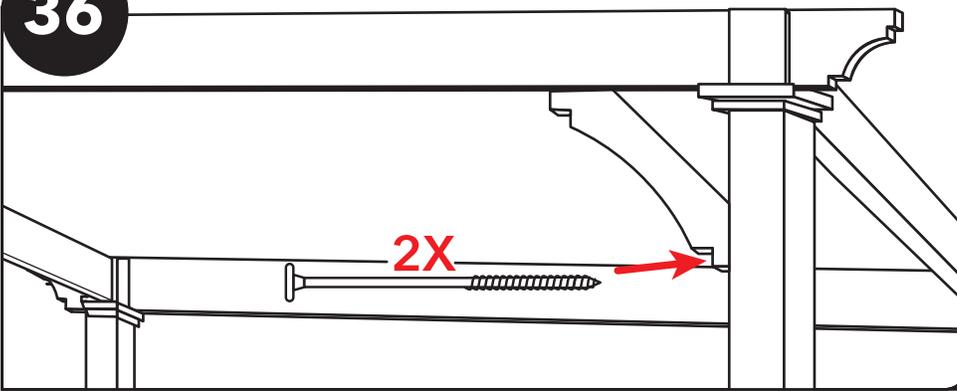
Keeping the brace flush with the outside of the post, attach the brace into the post through the pre-drilled holes with the 5" Timberlock screws.
