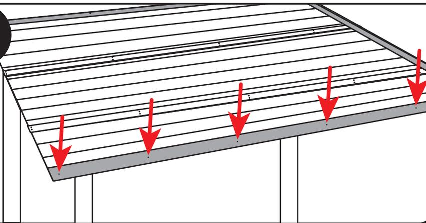
Install the back drip edge. Place drip edge on top of the lath. Keep flush with edge of roof. Fasten with one 1 1/4" stainless steel screw every 24" and one final screw at the end. Cut to size with tin snips.
