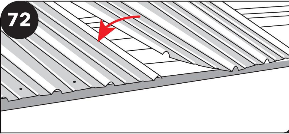
The next piece must properly overlap on the far edge. Attach with 1" roofing screws at the lath.
