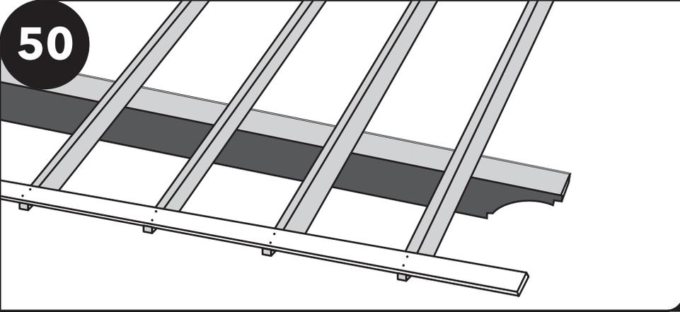
Place first board on low side of pavilion. Groove side facing away from the structure, tongue side facing toward the remaining boards.
