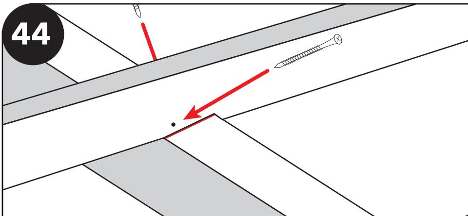
Attach rafter to high side header with two 3 1/2 " screws into pre-drilled holes. One on each side.
