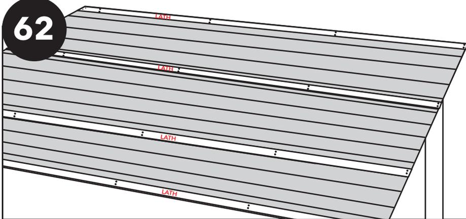
Repeat the process spacing each lath 20" - 24" apart. The last lath piece must sit 1/8" - 1/4" away from the edge of the roof decking.
