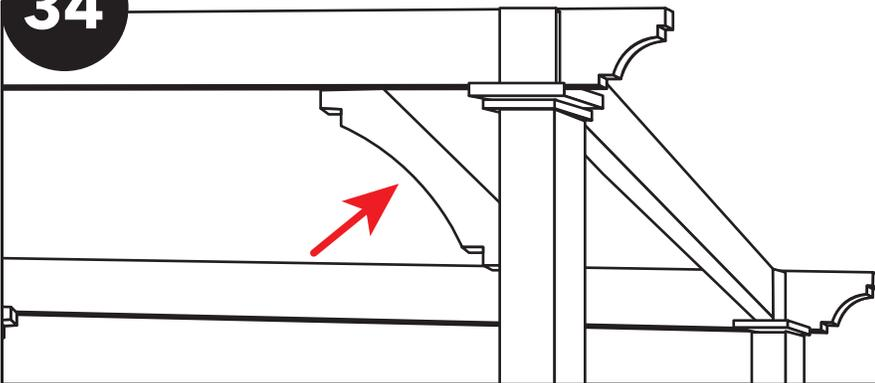
Hold the brace in place, being sure the top and bottom are flush with the header and the post and (for pressure treated: side attachment screws must face inward).
