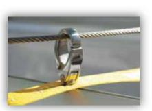
Infinity Canopy's hook and base instantly attach or detach the canopy to the cables and slide easily for a smooth movement. The hook can turn 90 degrees to lock the canopy to crossing cables and along with the base be used to connect two canopy sections end to end to increase the width of the canopy.
