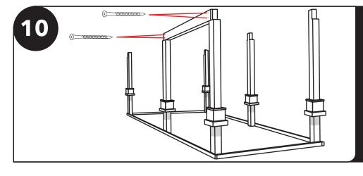
Starting with a corner post of the longest side and moving to the center post, attach first header with two 3 1/2" screws (not in pre-drilled holes) to hold header in place.
