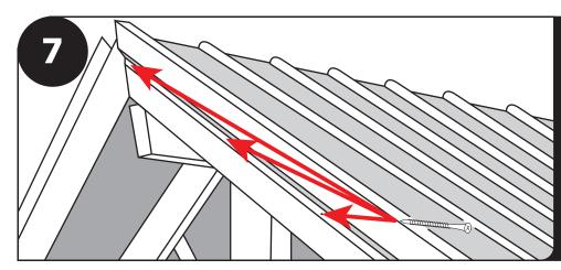
Once gable end trim is cut to angle, attach the trim piece with one 1" screw into the fascia board every 24" of the open gable end. Next, fasten the top of the same trim piece with 1" screws at every roof lath.
