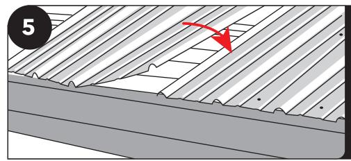
The next piece must properly overlap on the far edge. Last piece may need to be cut to size to be flush with the edge of the fascia.
