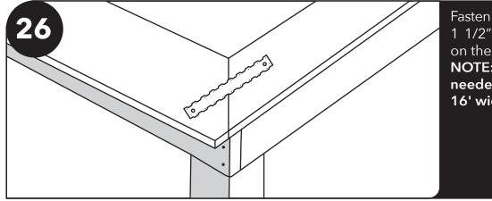
Fasten tie straps, ST2215, with 1 1/2" screws at every seam on the top of the plate.
