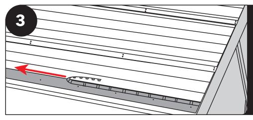
Install the ribbing roughly 1 1/2-2" from the bottom of the drip edge. Do not stretch the ribbing because the grooves of the roof must line up with the ribs.
