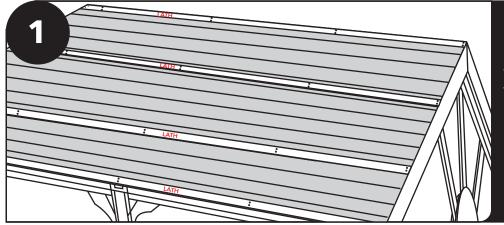
Fasten horizontal "Roof Lath" pieces with two 2" roofing nails at each rafter. Place the first piece of lath directly on top of the lowest decking board. Space each lath board roughly 20-24" apart with the longest piece placed at the bottom and the shortest piece at the top. (Lath boards may need to be cut to length.)
