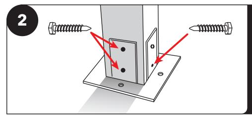
Screw into each post the remaining six 3/8" x 3" hex lags using the pre-drilled holes. Repeat with all posts.
