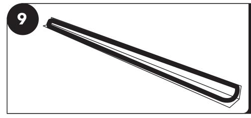
Locate ridge cap. Remove backing from foam and attach to the underside of the ridge cap. Place ridge cap, flush with previously installed trim, fastening every 24" with 1 1/2" screws on both sides.
