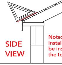
Note: With metal roof installation, fascia should be installed 3/4" higher than the top of the roof decking.
