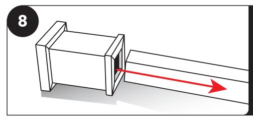
Slide your bottom post base on the post. Be sure to slide the bases up the post to make room for completing steps 9-22. NOTE: For HD High Wind brackets see the bracket appendices on page 21 (step 1) before moving on to step 9.
