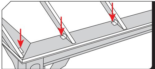
Fasten one "A23 Simpson" bracket to the side of each rafter with 1 1/2" screws. Then anchor the bracket to the plate with more 1 1/2" screws.
