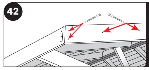
Fasten to the 2x4 rafter. One 2 1/2" screw at top and two at the bottom going into fascia. Then one every 16".
