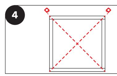
Once the template is in position, square the template. Do this by measuring diagonally from one corner to its opposite corner, then measure diagonally between the other two corners. These two dimensions **MUST** be the same. Adjust the template until the diagonal measurements are identical.
