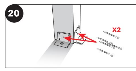
Make sure the posts are all level and everything is square. With base trim still raised, fasten two L-brackets on the outside edges of each post with five 2 1/2" screws per bracket. Some engineering specifications may require 4 brackets per post. NOTE: For HD High Wind brackets see bracket appendices on pages 21-22 (Steps 2-4.)
