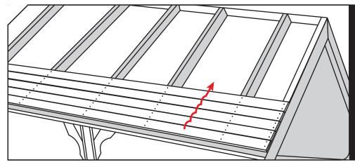
Securely interlock each piece of the roof decking, starting from the bottom and working up. Repeat step 33 on the remaining side of roof.
