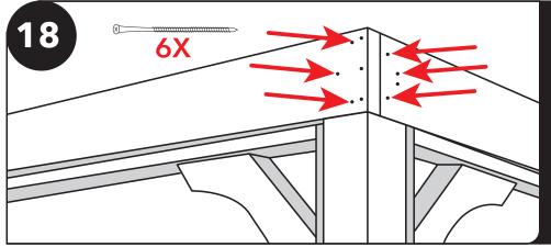
Locate 24 8" GRK screws in the hardware box. Those go in the pre-drilled holes at the corners of the beams. (6 per corner)
