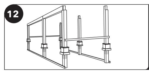
Remove template boards from the posts on the short side. Attach a template board spanning from the two corner posts on the short sides.
