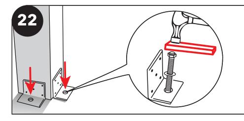
Before inserting the bolt, make sure dust is removed from hole. Then screw the nut and washer are on about 1/8" below the top of the bolt. Next, insert the wedge anchor bolt into the hole. To protect the threads and nut, tap the bolt into the ground with a piece of wood as a buffer.
