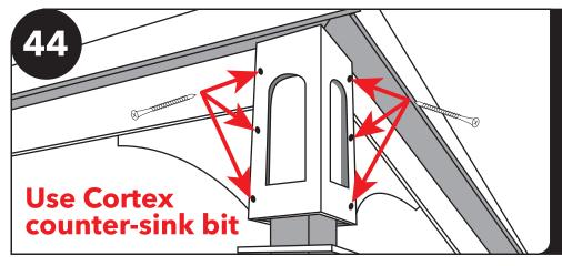
Place the outside corner trim box flush against the header and the brace, being sure that the top corner point is centered on the plate seam. Fasten with six 2 3/4" Cortex screws into the pre-drilled holes on the face of the corner trim.
