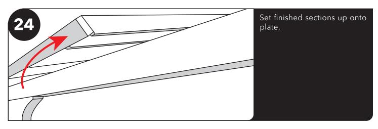
Screw the two sections together at the top with two 2 1/2" screws between every rafter. Keep ends even.
