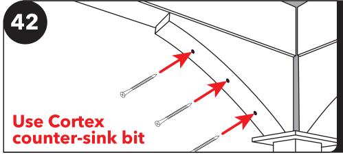
Install the bottom brace covers using three 2 3/4" Cortex screws. Continue with all 8 braces.
