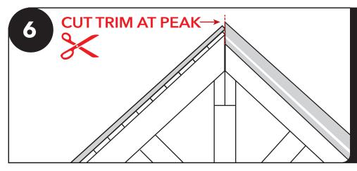
Once you have all the tin installed, hold the gable end trim in place to mark the upper end of the trim that will need to be cut to meet flush with the other side.
