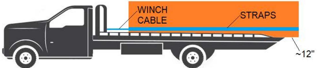
**Step 3:** Arrive at the drop-off location, back into the area, stop the truck. Tilt the bed of the truck up.
