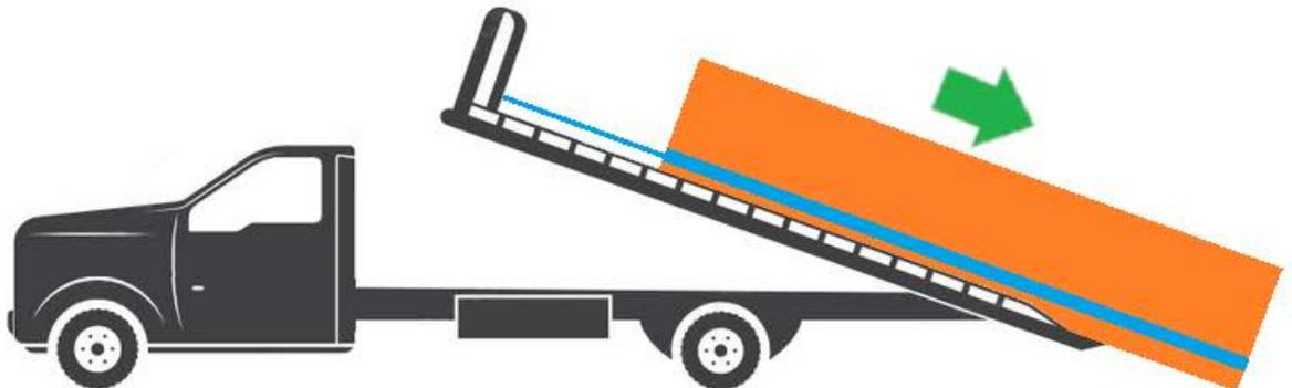
**Step 5:** Inch the truck forward while slowly lowering the crate until the crate is fully on the ground.
