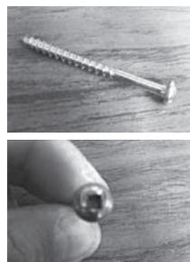
**18.** Following the layout pattern on the rafters begin installing the purlins across the top of the rafters using the steel deck screws. **NOTE:** The 2.5" stainless steel self-tapping purlin screws will be used on step #18 to attach the purlins to the each rafter. (Requires #2 square drive bit).
