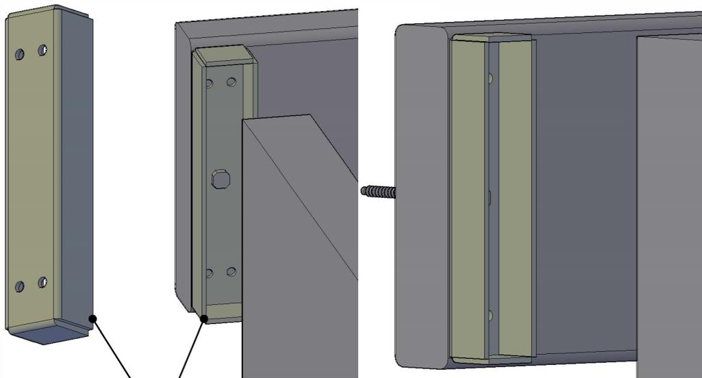
Flush Mount Rafter Bracket will recess inside open end of Rafter
