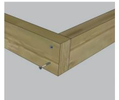
3. Connect the corners of the template pieces by driving two  $21\!\!\!/$  screws through the side of the template boards.
