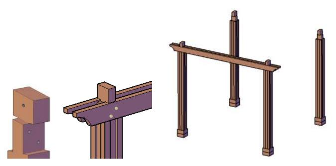
One the 2 supports have one large beam already attached or a few 18" pieces depending on size, this add support and strength to the structure. This beam must be in the interior of the support and bolted after you attach the supports to posts as shown below:
