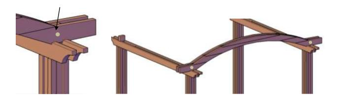
**Step 4.** Attach secondary knee brace to post & arched rafter with two bolts, washers & nuts. (Match numbers). Tap the bolt all the way into the wood to set it, then add a washer and nut and lightly tighten. *Repeat this step with the other end arched rafter.*
