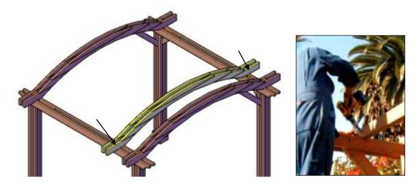
**Step 7:** Attach roof slats to rafters & with deck screws (1 5/8" x #8"). The roof slats are all notched identically. The roof slats are notched to fit into each other. Place the center roof slat first (the slat with groove on both sides) and then the rest for both sides.
