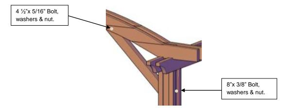
**Step 5.** Attach main knee brace to post & dual support beams with two bolts, washers & nuts. (Match numbers). Tap the bolt all the way into the wood to set it, then add a washer and nut and lightly tighten. *Repeat this step with the other main knee brace.*
