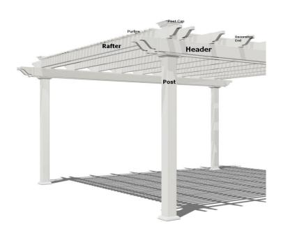
All units measure width x projection. These are on center post measurements, therefore will leave an overhang for the canopy. These are the extensions past the post center. See the overhang chart for the true canopy size. S:\USA Vinyl\Customer Service Sales\Selling Information\Outdoor Products\Pergolas\Width x Projection Diagram
