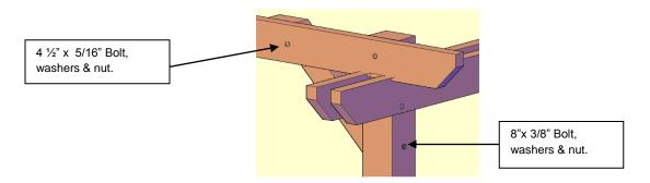
**NOTE:** if your pergola is with lattice roof , you will attach the secondary knee brace like this:
