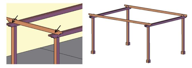
**Step 4.** Attach secondary knee brace to post & rafter with two bolts, washers & nuts. (Match numbers). Tap the bolt all the way into the wood to set it, then add a washer and nut and lightly tighten. *Repeat this step with the other end arch.*
