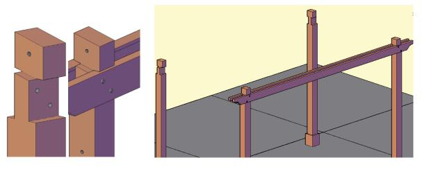
One the 2 supports have one large beam already attached or a few 18" pieces depending on size, this add support and strength to the structure. This beam must be in the interior of the support and bolted after you attach the supports to posts as shown below:
