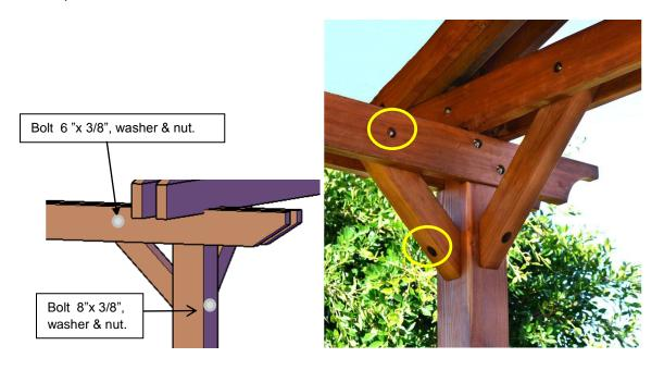
**Step 6.** Attach roof panels to rafters with post (6 "  $\times$  3/8") washers & nuts . Tap the bolt all the way into the wood to set it, then add a washer and nut and lightly tighten. The panels are all notched identically.
