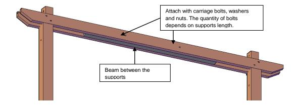
**Step 3.** Attach corner rafter to posts with one bolt per post (6 " x 3/8") washer & nut and use deck screws to attach the other rafters. (Match numbers). Tap the bolt all the way into the wood to set it, then add a washer and nut and lightly tighten.
