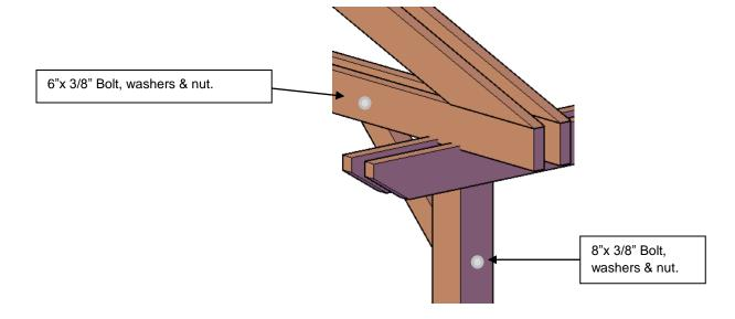
**Step 5.** Attach main knee brace to post & dual support beams with two bolts, washers & nuts. (Match numbers). Tap the bolt all the way into the wood to set it, then add a washer and nut and lightly tighten. *Repeat this step with the other main knee brace.*
