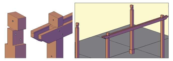
One the 2 supports have one large beam already attached or a few 18" pieces depending on size, this add support and strength to the structure. This beam must be in the interior of the support and bolted after you attach the supports to posts as shown below:
