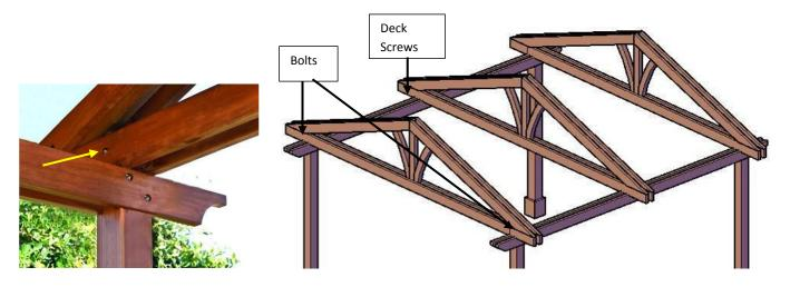
**Step 4.** Attach Secondary Knee Braces to post & rafter with two bolts, washers & nuts. (Match numbers). Tap the bolt all the way into the wood to set it, then add a washer and nut and lightly tighten. *Repeat this step with the other end arch.*
