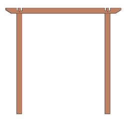
One the 2 supports have one large beam already attached or a few 18" pieces depending on size, this add support and strength to the structure. This beam must be in the interior of the support and bolted after you attach the supports to posts as shown below:
