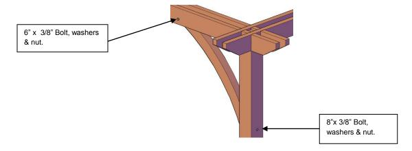
**Step 5.** Attach main knee brace to post & dual support beam with two bolts, washers & nuts. (Match numbers). Tap the bolt all the way into the wood to set it, then add a washer and nut and lightly tighten. Repeat this step with the other main knee braces.
