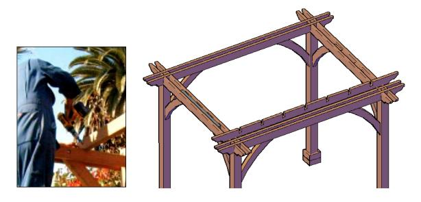
**Step 7.** Attach roof slats to roof slats and rafters with deck screws (3" x #8). The roof slats are all notched identically. The roof slats are notched to mesh with the roof slats. The rafter tops are marked in ink every 18 inches with 2 lines. Place one roof slat into the lines on one end and begin to attach. *And repeat the process in all roof slats*.
