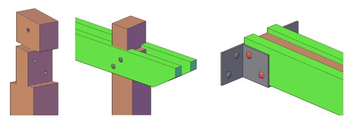
One the 2 supports have one large beam already attached or a few 18" pieces depending on size, this adds support and strength to the structure. This beam must be in the interior of the support and bolted after you attach the supports to posts as shown below:
