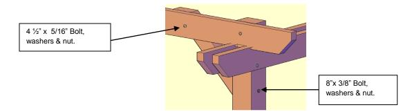
**NOTE:** if your pergola is with lattice roof, you will attach the secondary knee brace like this:
