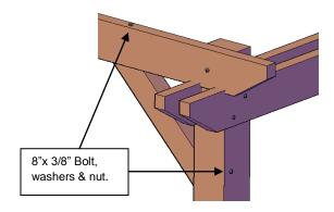
**Step 6.** Attach main knee brace to post & dual support beam with two bolts, washers & nuts. (Match numbers). Tap the bolt all the way into the wood to set it, then add a washer and nut and lightly tighten. Repeat this step with the other main knee braces.
