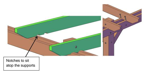
**Step 8.** Attach slats to rafters & with deck screws (3" x #8). The roof slats are all notched identically. The roof slats are notched to mesh with the rafters. The rafter tops are marked every 18 inches with 2 lines. Place one roof slat between the lines on one end and begin to attach. *And repeat the process in all roof slats*.
