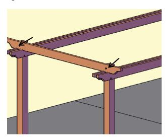
**Step 5.** Attach secondary knee brace to post & rafter with two bolts, washers & nuts. (Match numbers). Tap the bolt all the way into the wood to set it, then add a washer and nut and lightly tighten. Repeat this step with the other end arch.
