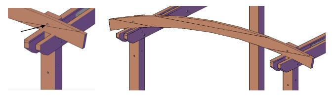
**Step 4.** Attach secondary knee brace to post & arched rafter with two bolts, washers & nuts. (Match numbers). Tap the bolt all the way into the wood to set it, then add a washer and nut and lightly tighten. *Repeat this step with the other end arched rafter.*
