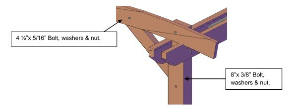
**Step 5.** Attach main knee brace to post & dual support beams with two bolts, washers & nuts. (Match numbers). Tap the bolt all the way into the wood to set it, then add a washer and nut and lightly tighten. *Repeat this step with the other main knee brace.*
